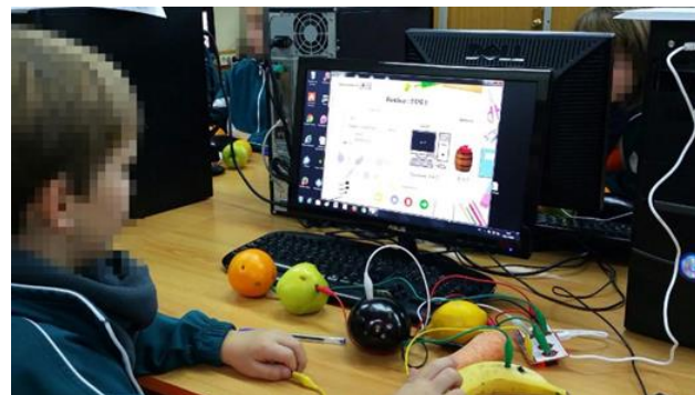
FIGURE 3. Child executing a snippet on PrimaryCode (left) and watching what happens to the outputs and variable (represented with a barrel), both on the right. In this case, the interaction is done with fruit connected through Makey Makey.
