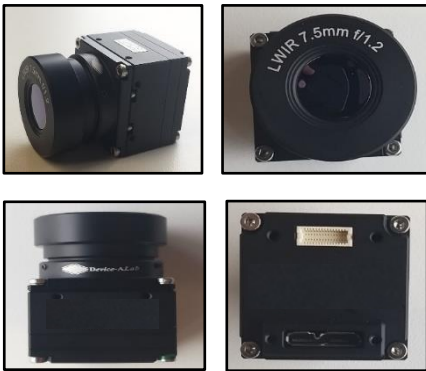
Fig. 7. Prototype thermal VGA camera model for acquiring local data
