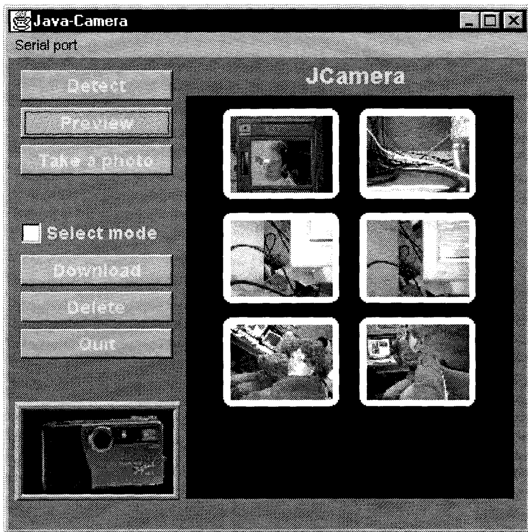
Fig 2: Example of a simple user interface & basic application software to download and manage the pictures from a digital still camera; this has been programmed using the generic API and camera classes described in this paper.
