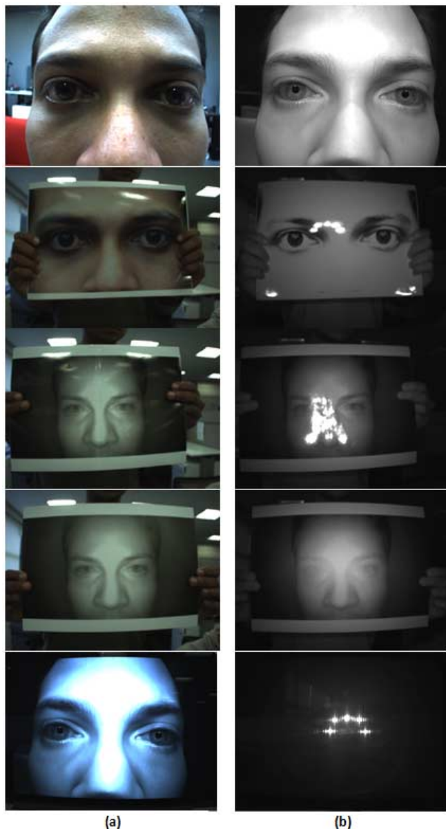
Fig. 4. Different Test Scenarios on the proposed system: (a) Visible Image, obtained by the system and (b) NIR Image acquired. First row is a live person. Second row is attack with a high quality visible printed image. Third row and fourth row are attacks with high quality NIR printed image (on two different photographic papers - glossy and matte). Fifth row is attack with NIR image shown in a laptop screen with high resolution retina display.
