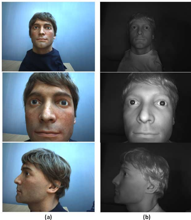
Fig. 5. An example for a sophisticated attack scenario: (a) Visible Image, obtained by the system and (b) NIR Image acquired. First row shows the realistic 3-D face model is used to test the presentation attack detection techniques. Second row is a close up look to indicate the human like skin, hair and ocular properties of the mannequin. Side view is shown in the third row.
