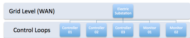
Fig 2(a): Legacy Electric Substation Architecture.
