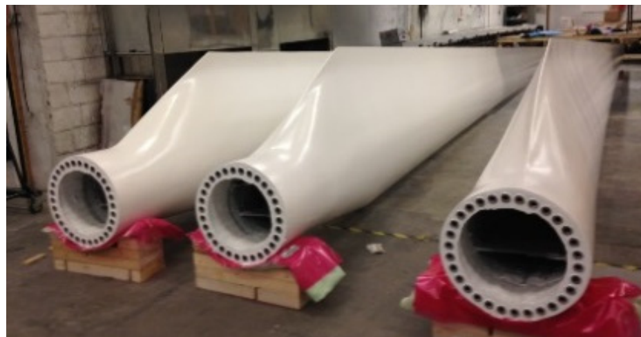
Figure 2. 13 m wind turbine blade after being manufactured and finished.
