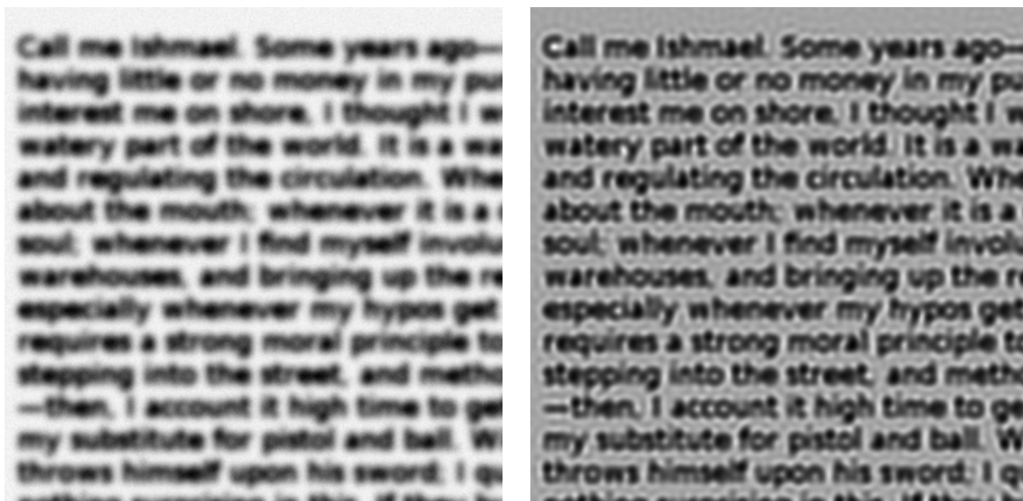
FIGURE 5.6: Low Noise Restoration with Unregularised Richardson-Lucy. Left: The Image, degraded by a known PSF and corrupted with a lower level of additive Gaussian noise than used in Figure 5.7. Right: Image restored with 128 iterations of unregularised Richardson-Lucy deconvolution with the known PSF. The steep discontinuity between the uniform background and solid text produces slight ringing artifacts that can be seen outlining each word. Noise amplification artifacts are more present over the uniform background than the text.
