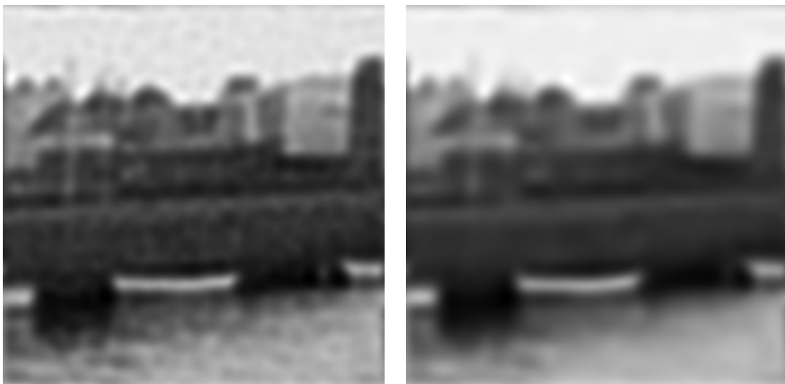
FIGURE 5.10: Unregularised and Wavelet-Regularised Richardson-Lucy Restoration. Left: Image restored with unregularised RL deconvolution. No ringing artifacts present, due to the lack of extremely sharp discontinuities in the original image, but noise amplification artifacts are clearly visible, and ringing artifacts would emerge with further iterations.
