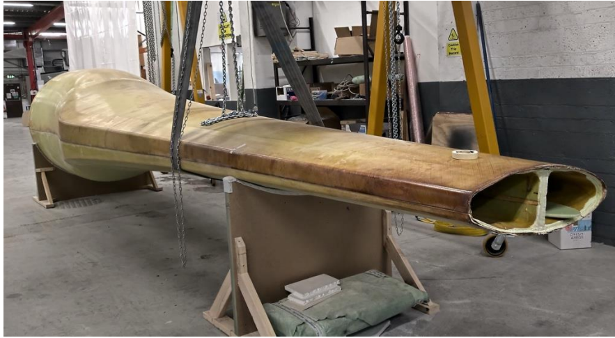
Figure 1. The main body of the tidal turbine blade (manufactured at ÉireComposites).
