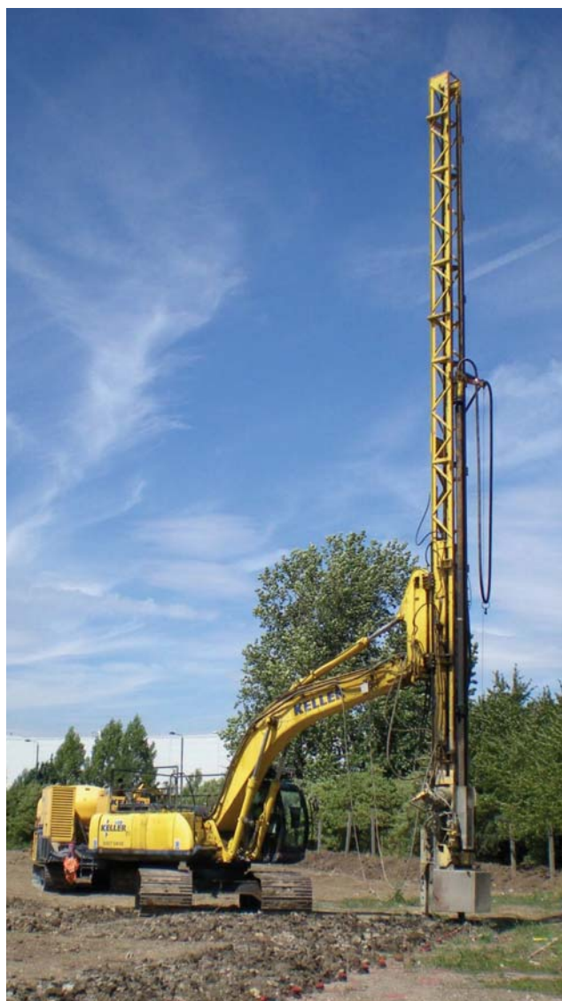
Figure 1. Keller Geotechnique's DDSM rig
