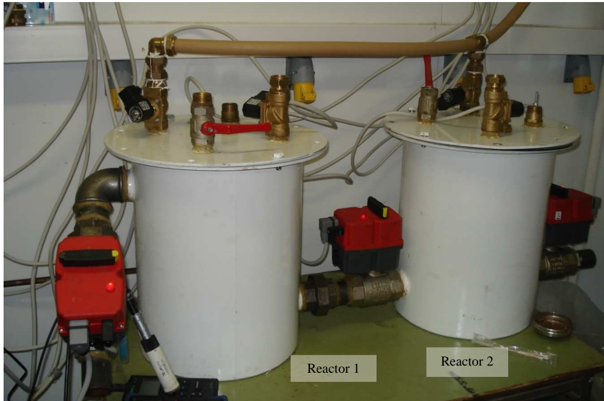
Figure 3.1 - Pilot scale ASF-BR commissioned within a temperature controlled room of the Environmental Engineering laboratory, NUI Galway.
