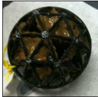
Figure 4.6 Media with thick biofilm accumulation
