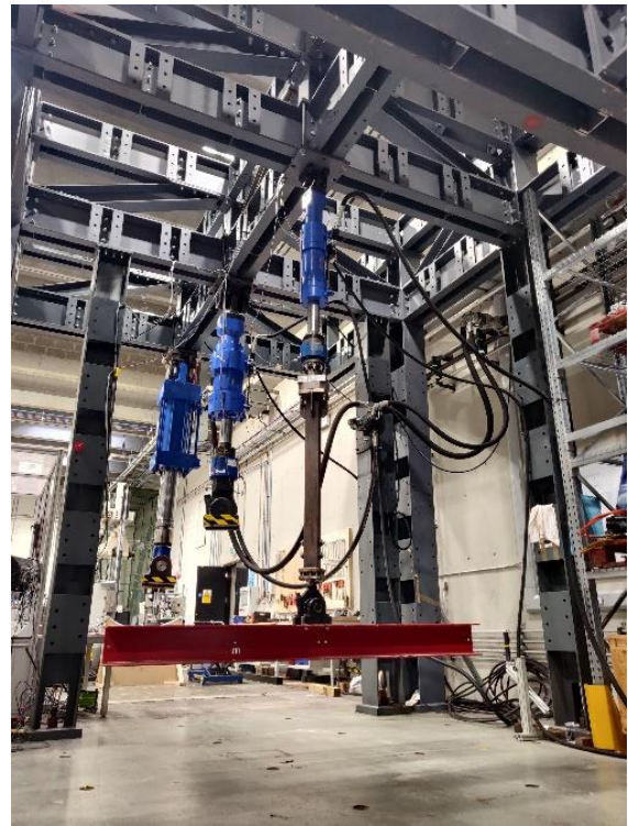
Figure 3. A sample installation of hydraulic actuators at the Large Structures Test Laboratory, NUI Galway.
