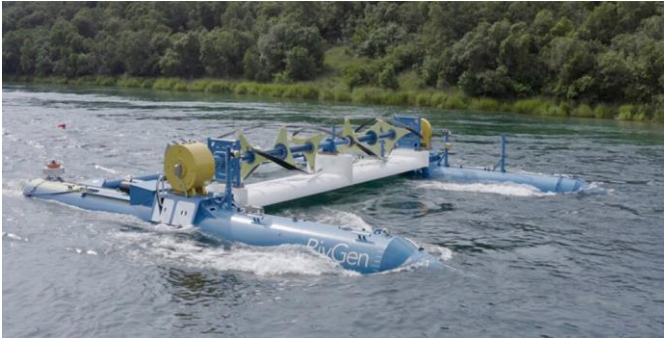
Figure 4. RivGen power system on-site, ready for commissioning in Igiugig, Alaska [6]
