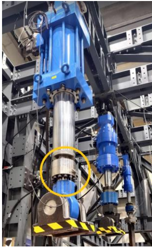
Figure 6. In-line load cell mounted on a hydraulic actuator at the Large Structures Test Laboratory, NUI Galway
