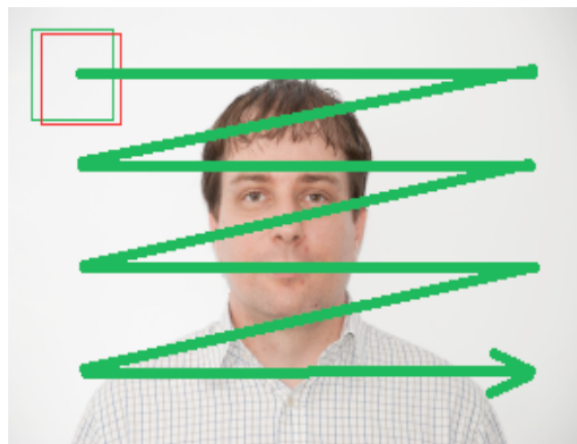
Figure 2: Face detection scans each image frame; in practice the entire image frame does not need to be scanned if a-priori data can be used to predict where the face will be found in the current frame.
