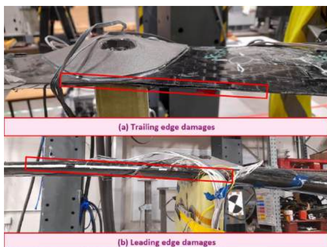
Fig. 7. Leading and trailing edge damages [13]
