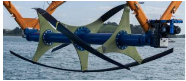
Fig. 2. Prototype turbine developed for towing tank and sea trails, image courtesy- ORPC
