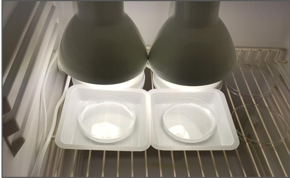
Figure 3.11. Experimental set-up for photoreactivation analysis using compact fluorescent lamps (OSRAM model DPRO MITW 23 W/840 E27).
