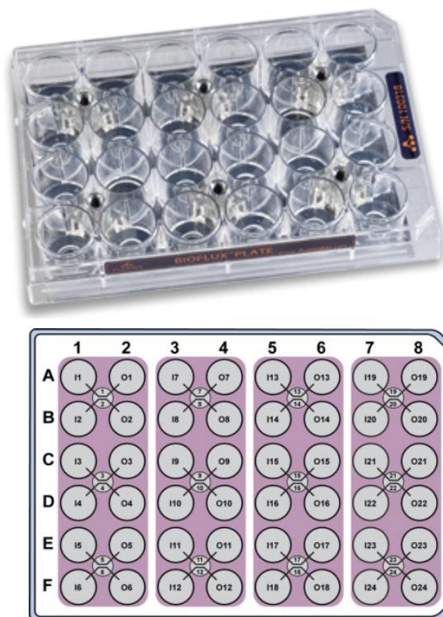
Fig. 2.1. Photograph and illustration of the 48-well plate used in the BioFlux 1000Z microfluidic system. Illustration demonstrates the input (left side, labelled “I”) and output (right side, labelled “O”) wells in each of the columns with the microfluidic channels (labelled 1-24) connecting the input and output wells. Images adapted from the BioFlux website http://fluxionbio.com/bioflux/ .
