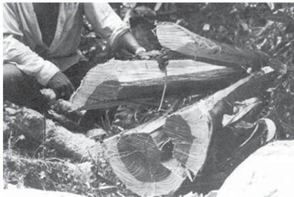
Figure 2. An intact Wapa tree is under extremely high levels of residual stresses that help to maintain its ideal mechanical conditions. When the Wapa tree is cut, the release of residual stress can cause the tree to burst apart. (Image source: http://www.fao.org .)
