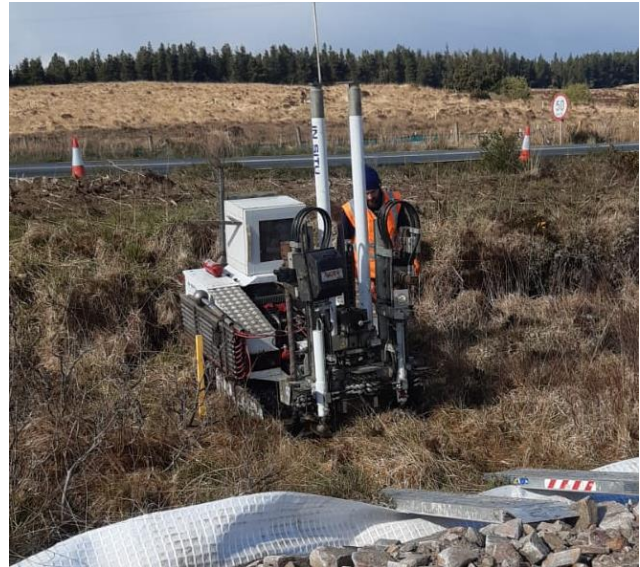
Figure 4. Lightweight CPT rig using ball-cone apparatus
