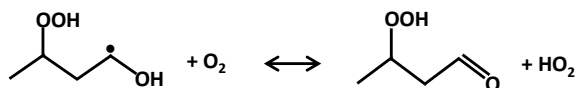
Figure 10: \alpha -hydroxy-hydroperoxyalkyl radical and its interactions with \text{O}_2 to form a carbonyl-hydroperoxide (e.g. hydroperoxy butanal) and \text{H}\ddot{\text{O}}_2 .
