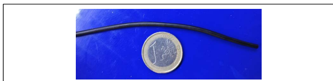
Fig. 2. Example of the 3D printable TMM filaments.
