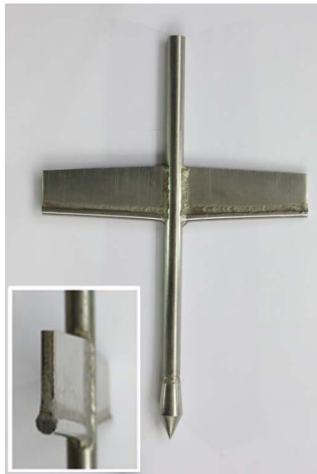
Figure 3. 150 mm-wide scale PIRT penetrometer (inset: wing profile with its 6 mm dia. leading edge bulb)
