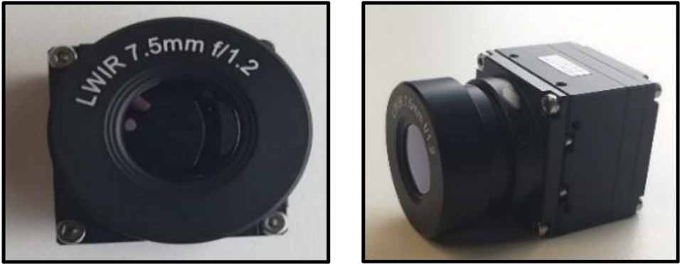
Fig. 5. Thermal LWIR camera sensor used for acquiring data locally in lab environment.
