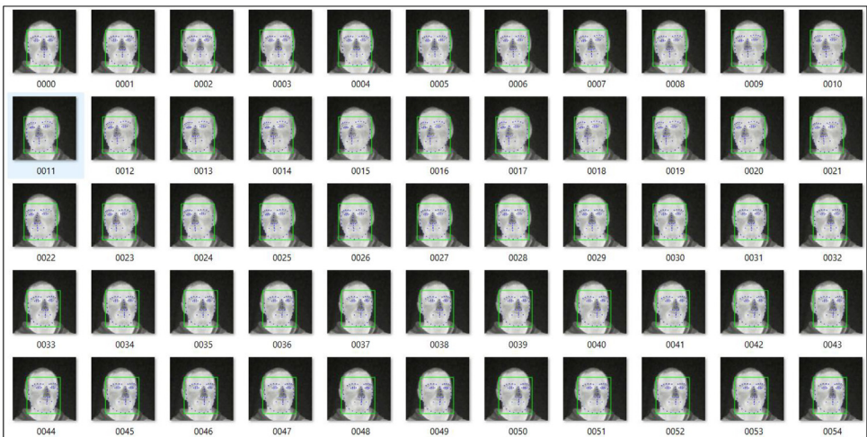
Fig. 11. Facial landmarks extracted using thermally tuned landmark detector [11,10] for finetuning canonical keypoint detector L.
