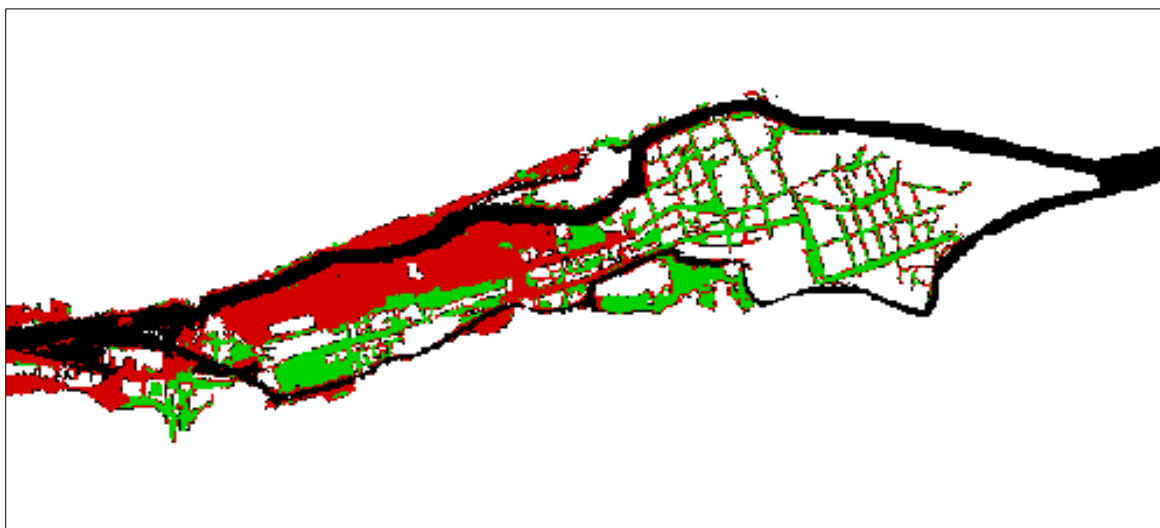
Figure 14. Map of inundation due to 50-year (red) and 200-year (green) joint coastal and fluvial flooding.
