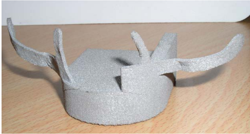
Figure 9: prosthesis model manufactured by solid freeform fabrication of titanium
