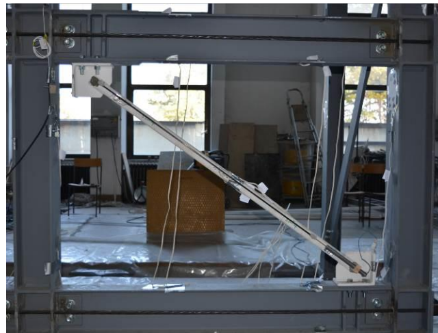
Fig. 9 – SHS brace and gusset plates
