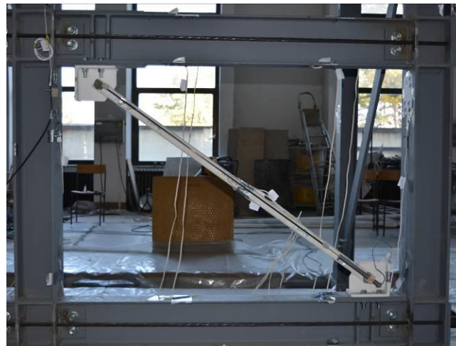
Fig. 9 – SHS brace and gusset plates
