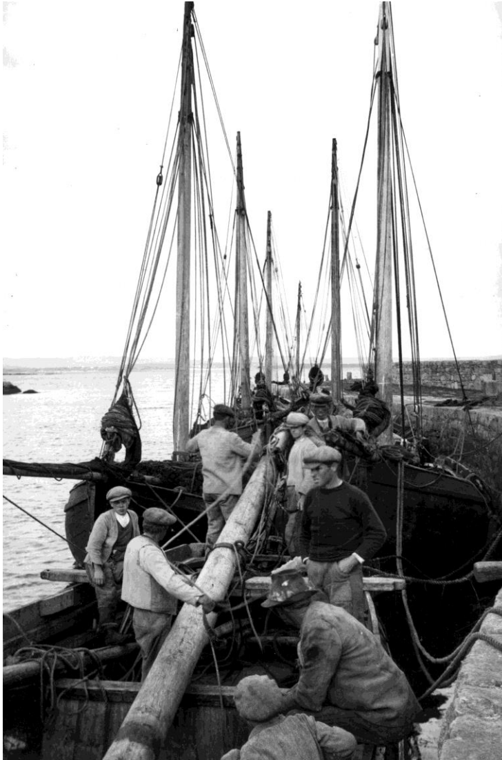
Figure 5.2 The hooker fleet at Máimín, Leitir Moir, about 1943. A crew is about to step the mast. (Scott, 2004, p.26) Used with permission from Fáilte Ireland.
