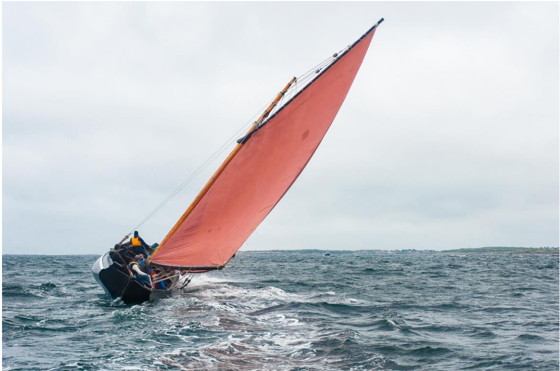
Figure 5.3 An Mhaighdean Mhara still going strong. Note the very large Tumblehome (apple-cheek-like rounded sides) creating a large cargo area. (Petroni and Dossena, 2017, p.68). Used with permission.
