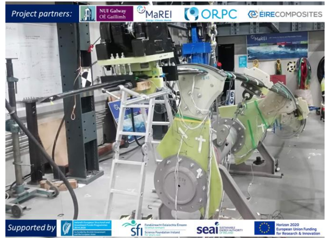
Fig. 6 A helical foil installed at the Large Structures Testing Laboratory undergoing structural testing using two actuators.
