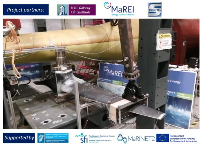
Fig. 4 A small tidal blade installed at the Large Structures Testing Laboratory undergoing structural testing using a single actuator.
