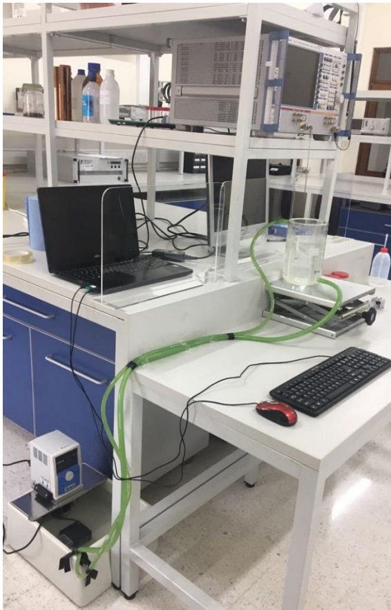
Figure 1. Experimental setup using a slim-form probe directly connected to the VNA. Blood samples were maintained at 37°C by pumping heated water from a large water bath to a temperature-controlled beaker. The beaker was then brought to the probe by a lifting platform, thereby minimizing uncertainties introduced by movement of the probe.
