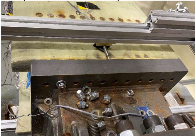
Figure 11. Failure of the T-bolt connectors.
