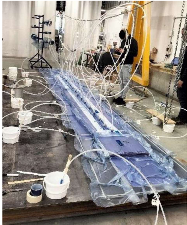
Figure 3. The vacuum-assisted resin transfer moulding process (for the spar cap).
