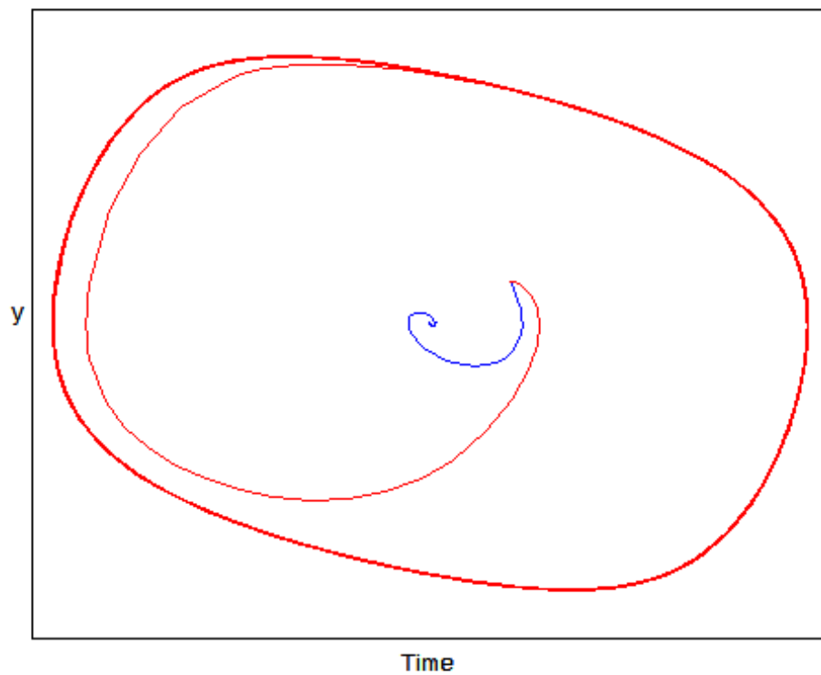
Figure 4: Stable Focus ( \lambda < 0 ) and Stable Limit Cycle ( \lambda > 0 )
