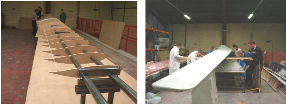
Figure 7. Construction of 12.6m wind turbine blade pattern
