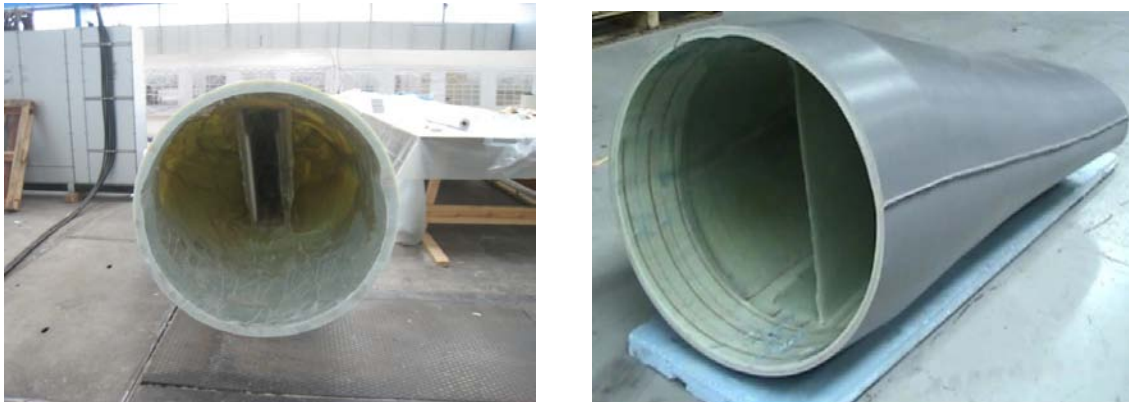
Figure 10. 12.6m glass fibre/epoxy wind turbine blade manufactured on electrically-heated ceramic composite tooling, showing (left) an internal view of the full blade; and (right) a section of the blade showing an in-mould UV-resistant coating
