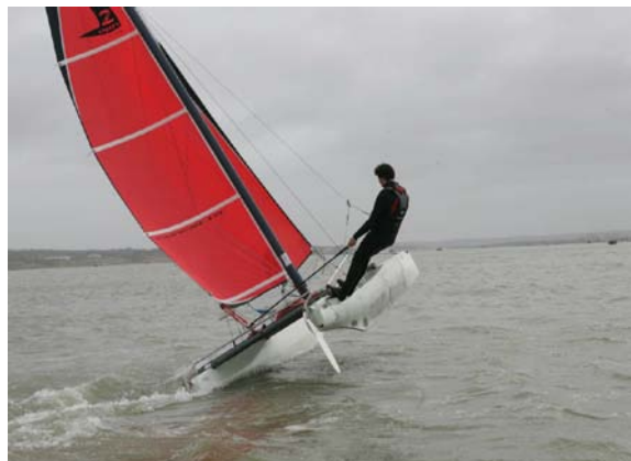
Figure 2. Sailing catamaran with GF/PP hulls, manufactured using the configuration in Figure 1.
