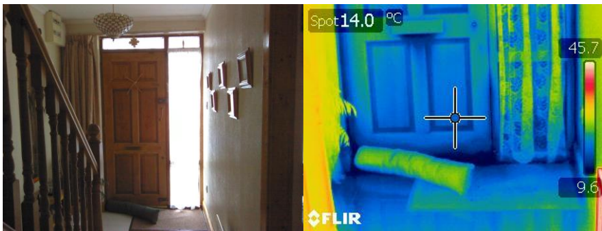
Figure 4. The thermal bridging experienced at the front door of a house constructed in 1994
