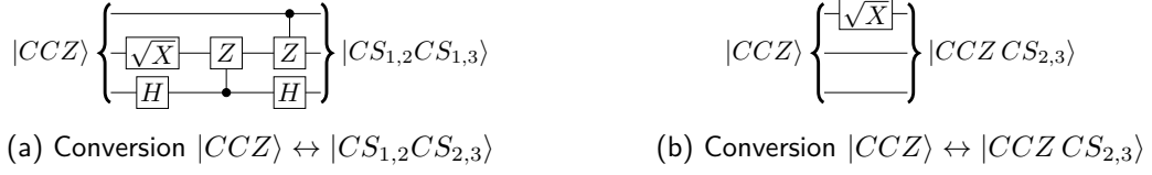
Figure 12: Two way conversion of resource states from [30]. These circuits are useful subroutines for some of our results.
