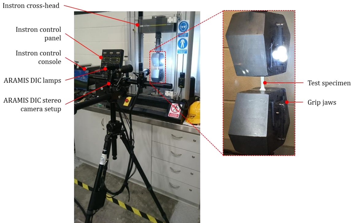
Figure 2: Instron 4467 uniaxial test equipment and ARAMIS DIC test setup.
