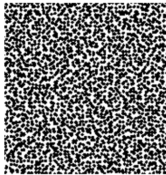
Figure 4: Computer-generated DIC speckle pattern printed with speckle diameter of 0.1 mm and 65% coverage.
