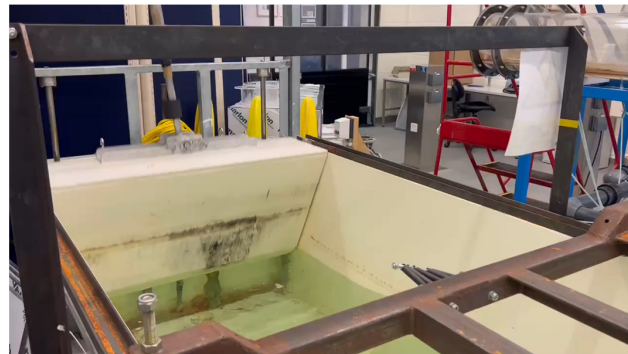
Fig. 1. Image of the wedged-shaped plunger-type wavemaker in the Hydraulic and Aerodynamics Laboratory at the University of Galway.
