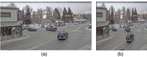
Fig. 15. Object shape distortion when (a) Aspect ratio is preserved and (b) Aspect ratio is not preserved.
