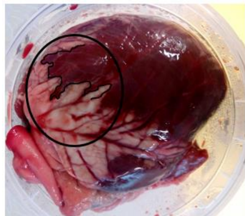
FIGURE 3. Lamb heart sample used to conduct dielectric measurements aimed at confirming the sensing radius calculated numerically. The area where measurements were performed is surrounded by a black circle and, within that area, the fat/muscle interface is marked.
