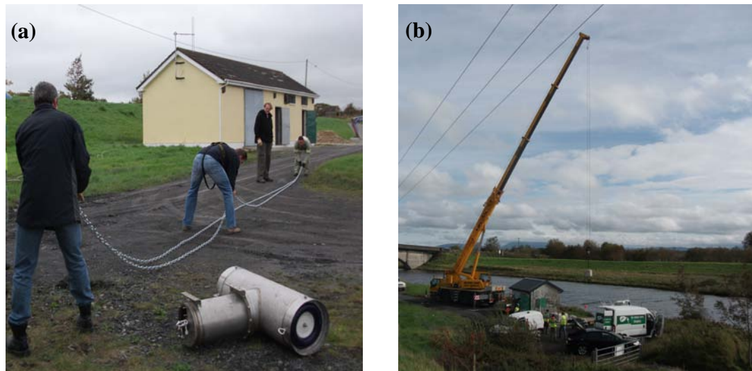
Fig. 5.3 (a) Preparation of the infrasound projector (right foreground) and (b) deployment of the infrasound projector from a crane at Clonlara.
