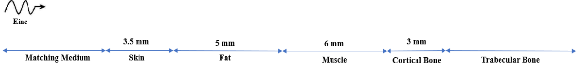
Fig. 2 The 1-D planar layered model of the human heel, which is composed of five layers: skin, fat, muscle, cortical bone, and trabecular bone. E_{inc} is the probing wave
