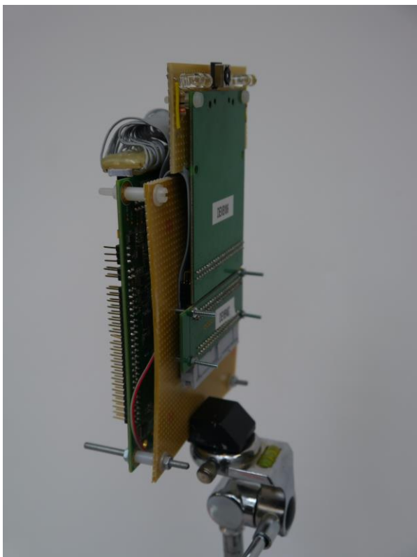
Fig. 4. Prototype device – side view. Smartphone form factor optics can be observed.
