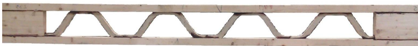
Fig. 1. Manufactured latticed LVL-webbed I-joist
