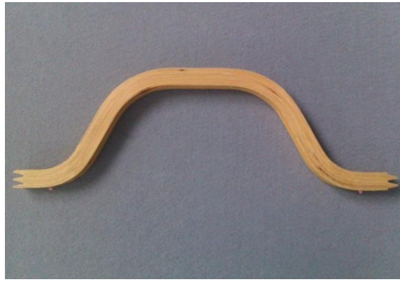
Fig. 3. Manufactured lattice web component with finger joints.
